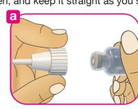
• If the needle is not kept straight while you attach it, it can damage the rubber seal and cause leakage, or break the needle (See Figure b).
